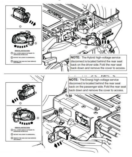
**NOTE:** Wait 5 minutes after the service disconnect plug is removed before continuing service. This allows any residual voltage in the high voltage system to dissipate.
