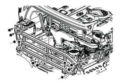
13. Disconnect and remove the traction battery fan.
