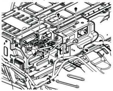
28. Remove the Traction Battery wiring cover.
